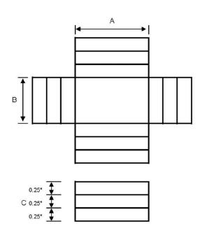
Each 0.025" section can be easily broken away to Create shield heights of 0.25", 0.50", or 0.75"
